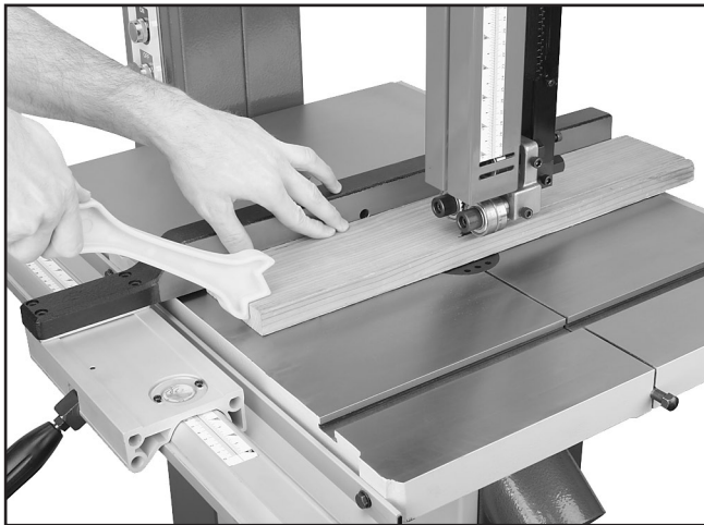
Figure 43. Ripping with a push stick.
